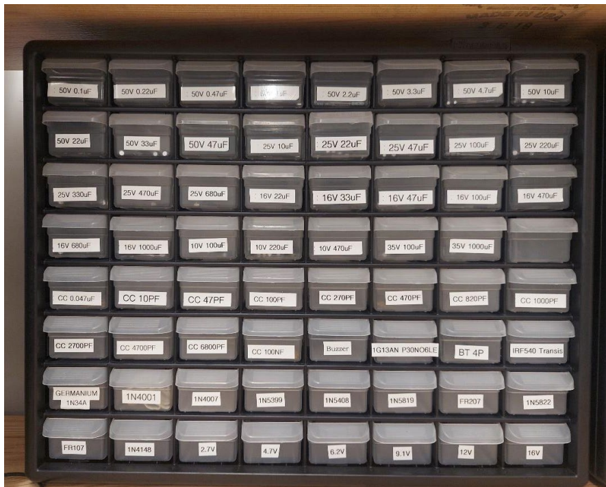
Figure 84: Bin organizer in Engineering Classroom W-182. The capacitors are arranged from lowest to highest value.
