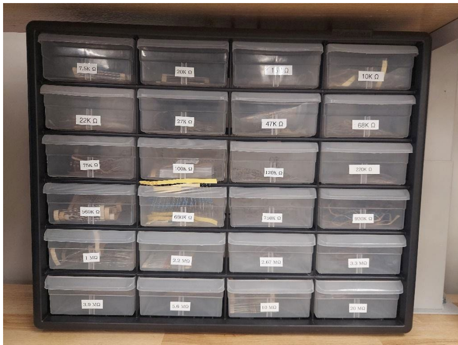
Figure 82: Bin organizer in Engineering Classroom W-182. The resistors are arranged from lowest to highest value.
