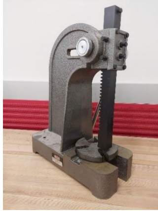
Figure 46:3-Ton-Arbor Press in the Machine Shop.
