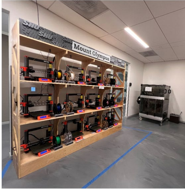
Figure 5: 3D printing room has 12 Prusa machines, 4 Ultimakers, and 1 Gigabot to allow for a variety of 3D printing experiences.
