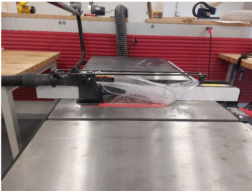
Figure 97: Sawstop safety table saw in Machine W-176 lab
