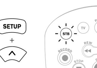
**5** When successfully paired, the green RF Adapter LED will stop blinking and will stay on.
